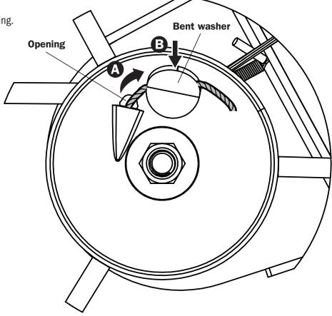
Attach & tighten the cable clamp on the cable. Leave about 1/2" extension of cable.
